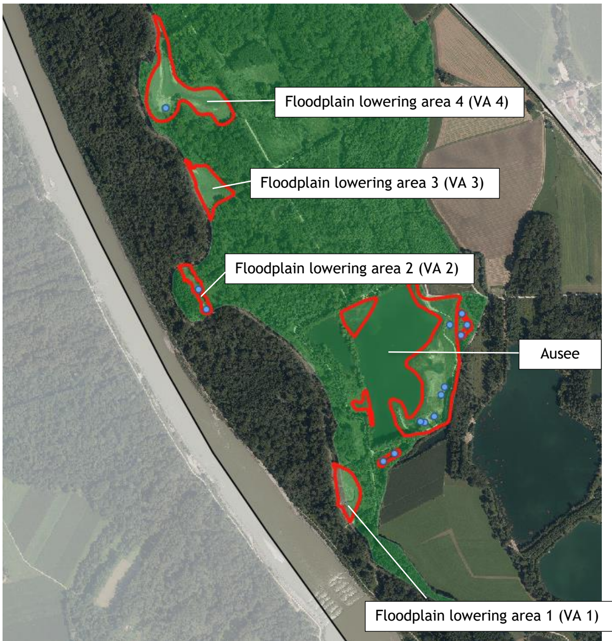
Figure 14: Action areas/construction zones in the Weitwörther Au (red), new amphibian water bodies (blue); LIFE-project area (green); ortho-photo Province of Salzburg
