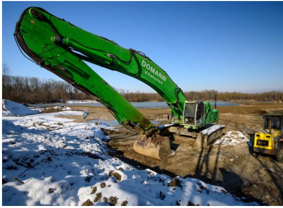
Figure 19: A long reach excavator used for shaping the shallows at Ausee (left). Dumping into Ausee was a challenge for the construction companies owing to difficult weather and soil conditions (right, photos: Ragger/REVITAL).
